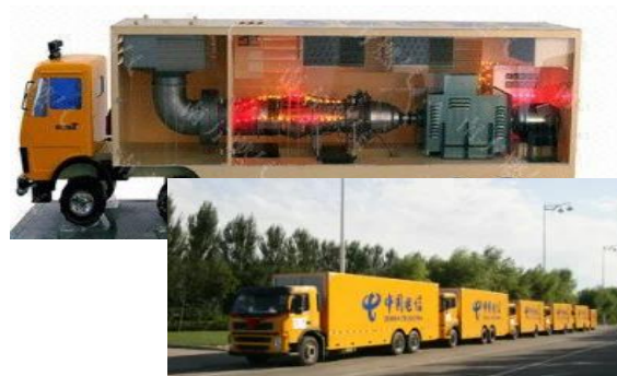
Mobile gas turbine generators – China
