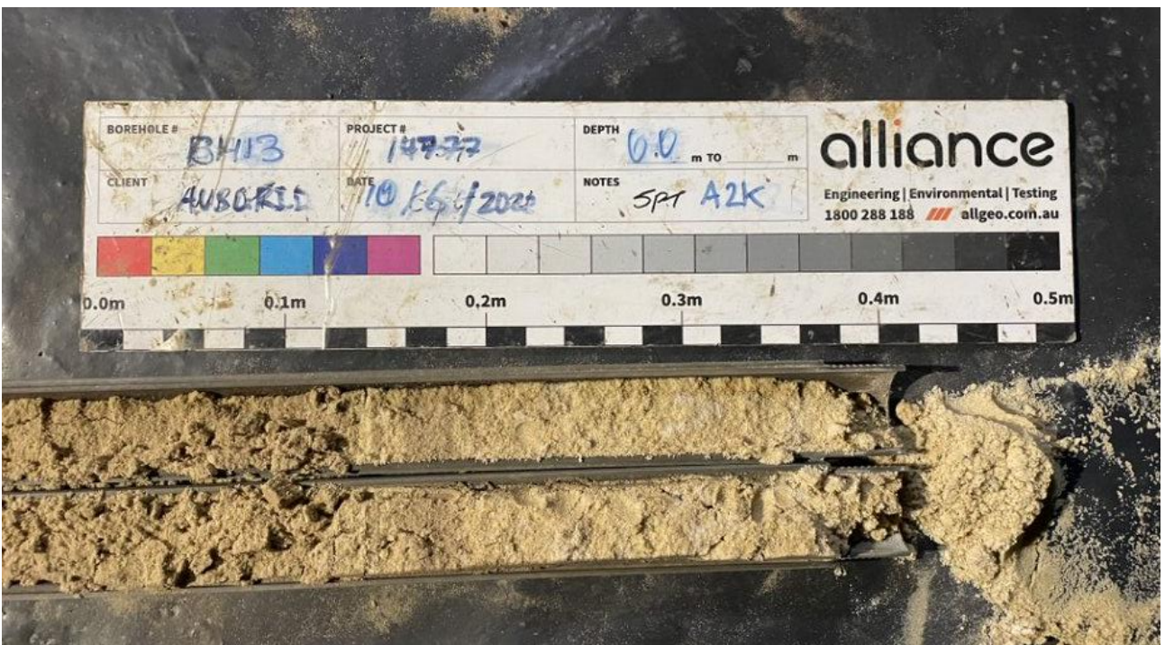
Photo 2 – SPT Split Spoon sample retrieved from borehole A2K-BH13 at 6.0m depth bgl
