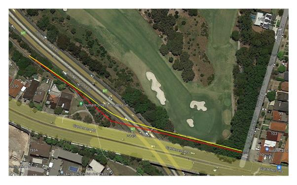
Figure 1-3 Horizontal Directional Drilling locations adjacent to Southern Cross Drive. Option 1 in Red and Option 2 in Yellow.
