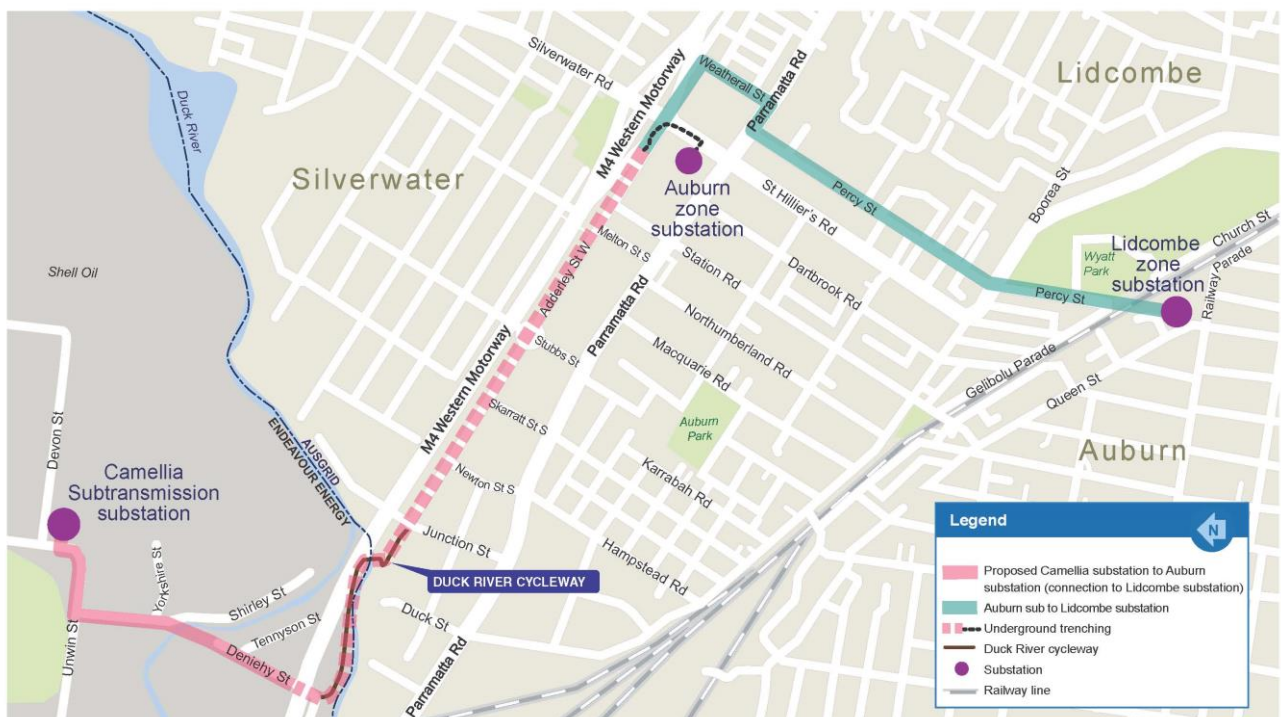
Figure 1 – Camellia to Auburn cable route
