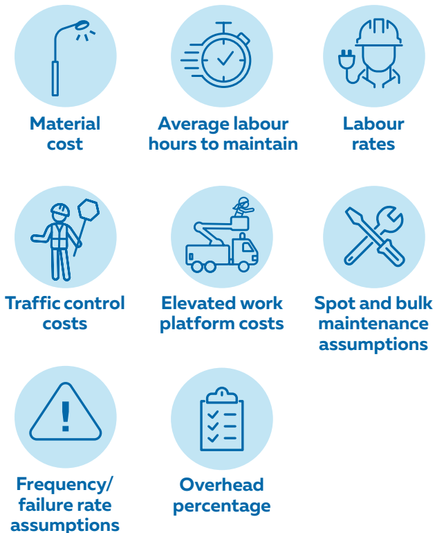
Figure 7 Inputs for calculating maintenance charges
