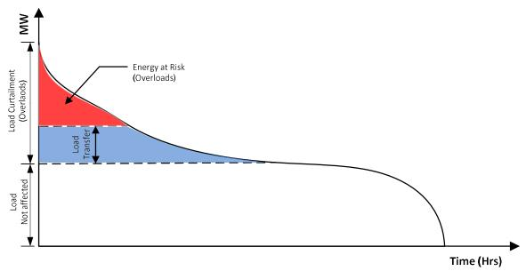
Figure 4-1: Illustration of Load Curtailment
