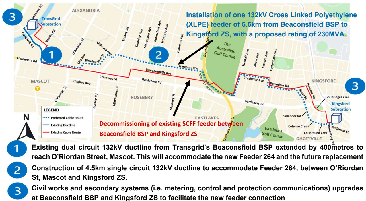
Figure 3-1 – Existing and proposed route of feeder 264
