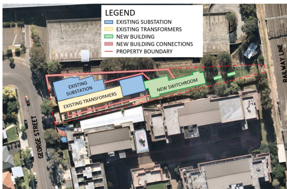
Figure 6-1 – Concept design arrangement showing the location of the new switchroom at Concord zone substation
