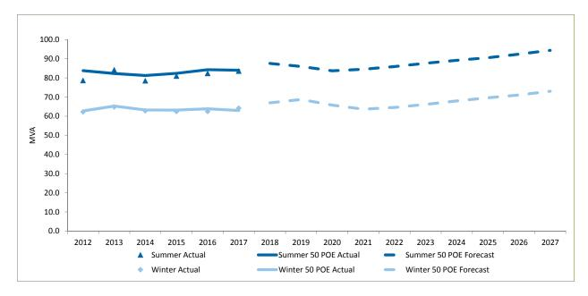
Figure 1 – Maximum demand forecast at Flemington zone substation
