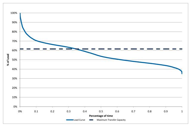
Figure 4 – Flemington Zone Substation Load Duration Curve (May 2016 to April 2017)
