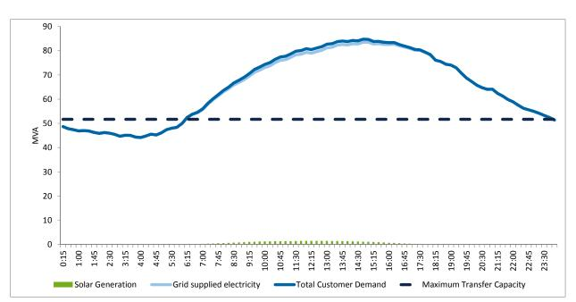
Figure 5 – Summer maximum demand profile at Flemington zone substation with maximum load transfer
