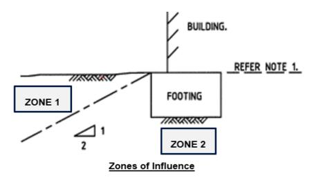
Zone 1: Excavation with shoring as normally required is acceptable.
