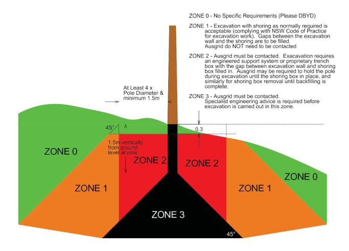
If your excavation is in the vicinity of any Ausgrid assets or structures, consideration shall be given to the risk of impacting on the stability of the structure. Such risk needs to be assessed by a competent person such as a civil engineer and any proposed support system shall be approved by Ausgrid.
