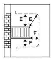
These dimensions apply if the height of the railing (or similar) plus distance E is greater than distance D
