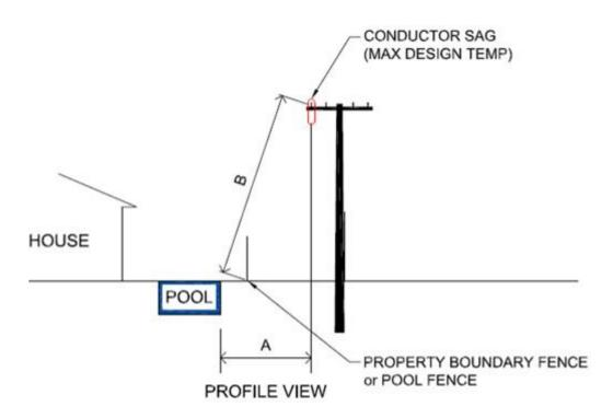
CLEARANCES BETWEEN SWIMMING POOL AND OVERHEAD CONDUCTORS.
