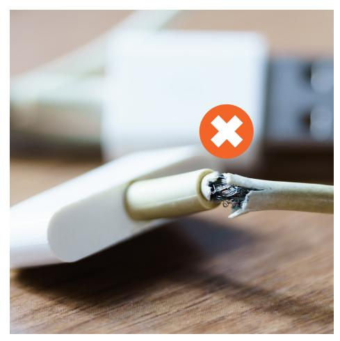
I only use electrical appliances with **undamaged** power cords.
