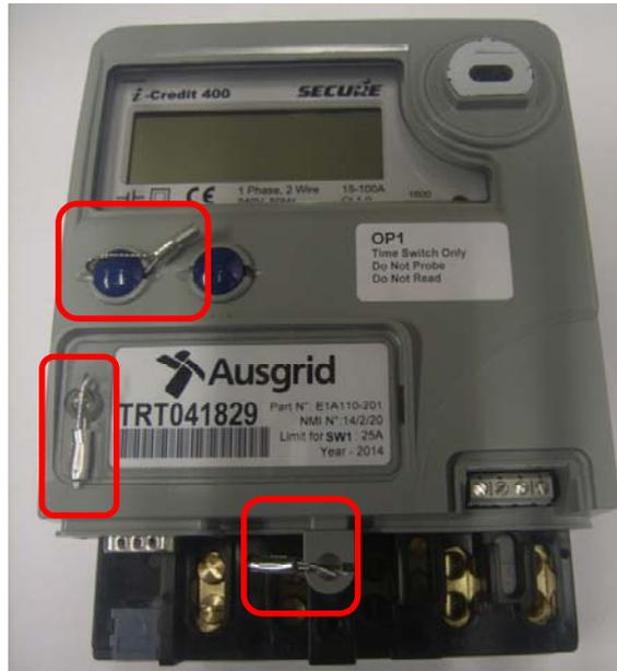
**Figure 8.4-7 Seals that must remain intact**
