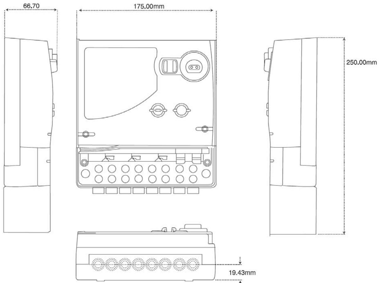
**Figure 6.2-3**The dimensions of Sprint meter
