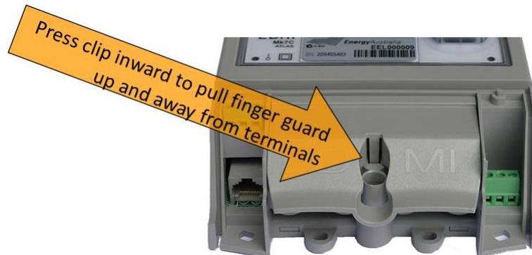
The finger guard must be reinstated after conductors are securely terminated
