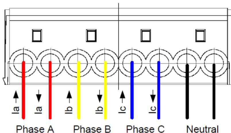
Figure 6.1-7: EET Mains Connection diagram
