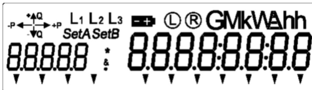
Figure 5.5-6: ECP Display – Test Pattern
