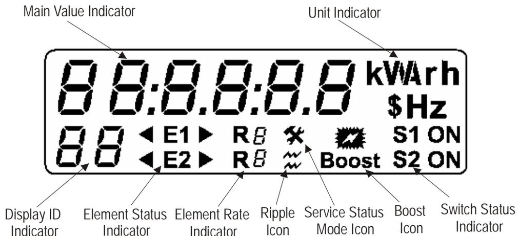
**Figure 4.2-6 i-Credit 400 meter display**
