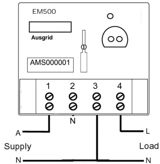
Figure 2.1-4 EM500 meter wiring schematic
