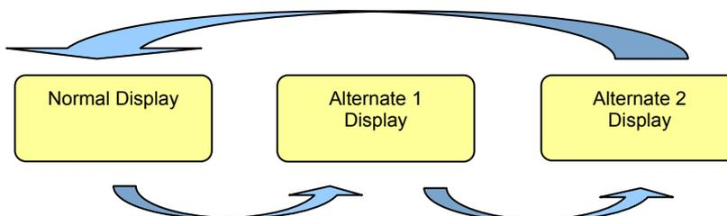
**Figure 5.4-8: Sequence followed by pressing and holding Display Select button**
