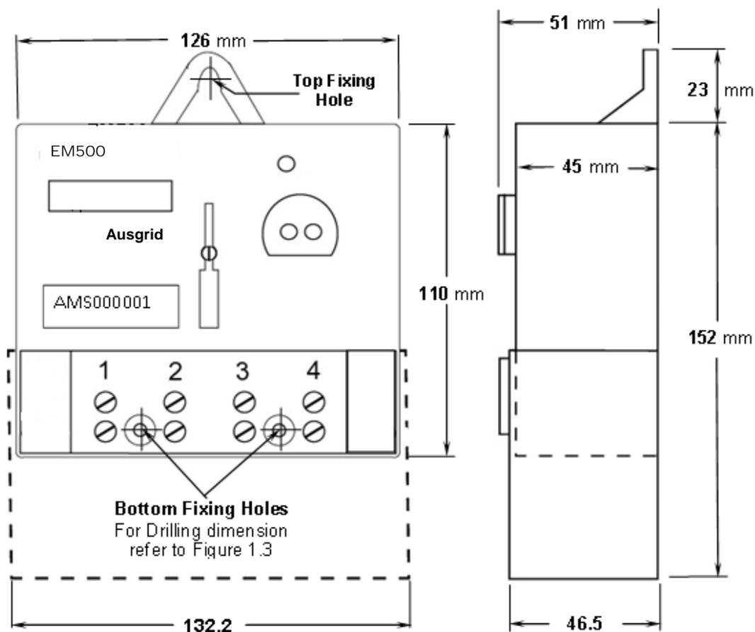
**Figure 2.1-2: EM500 meter dimensions and mounting diagram**
