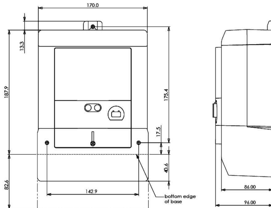
**Figure 5.4-2: LGC meter dimensions.**
