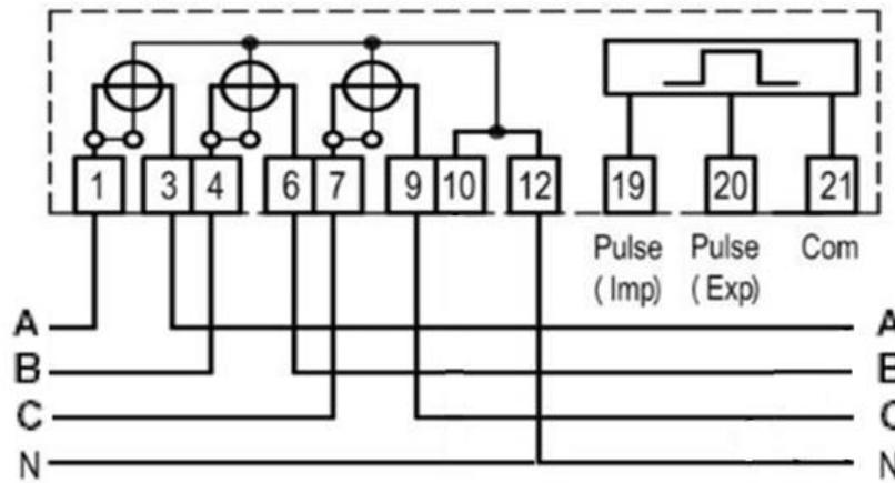
Figure 3.2-4 HLE meter wiring schematic
