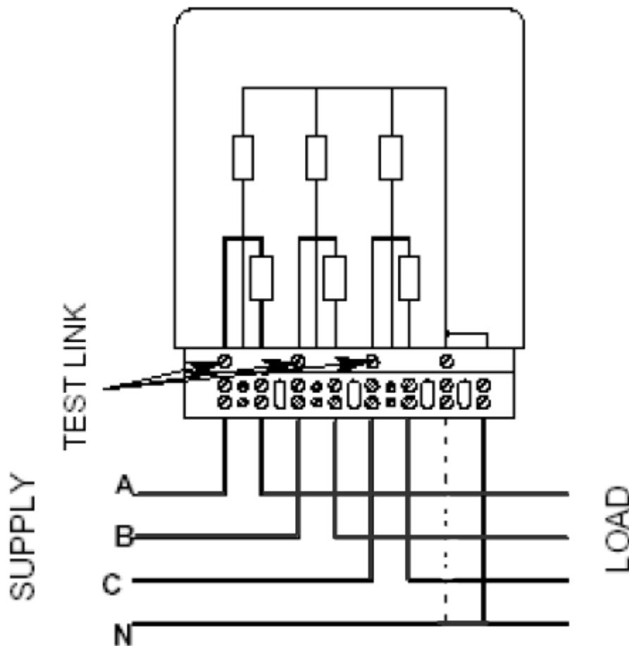
Figure 3.1-5 AMT meter wiring schematic
