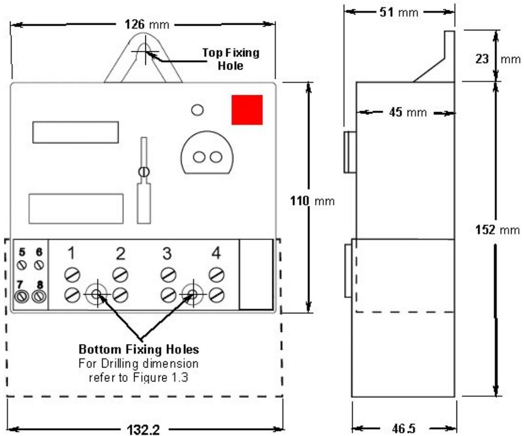
**Figure 4.1-3 EM1000 meter dimensions and mounting diagram**
