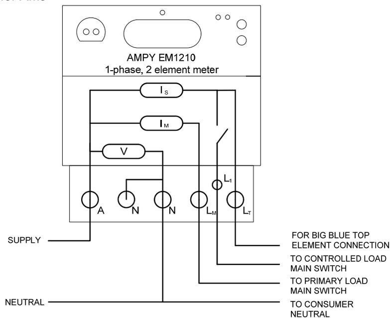
**Figure 5.2-4 Wiring Schematic for Standard Configuration - Structure 20**
