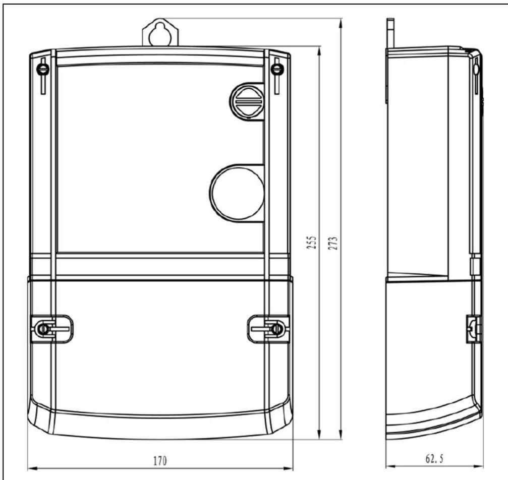
Figure 3.2-2 HLE Meter dimensions
