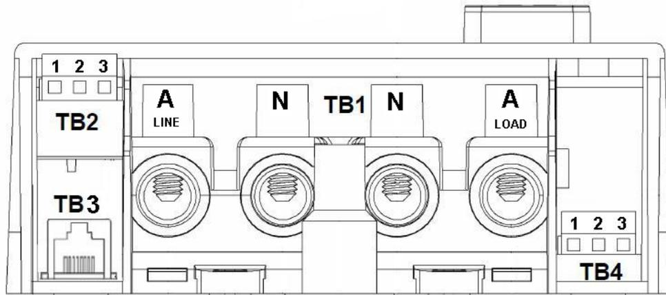
**Figure 4.3-6: EEL terminal block diagram**
