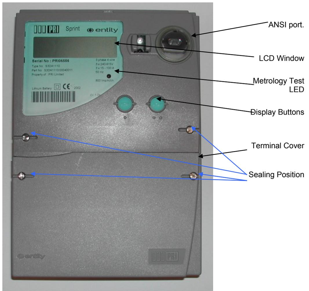
**Figure 6.2-2 Parts Identification**
