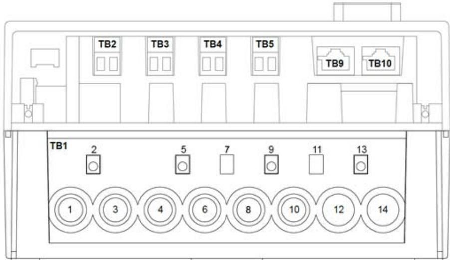
**Figure 5.5-4: ECP Terminal Identification**
