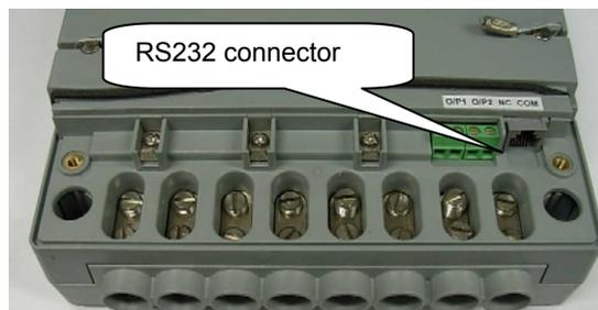
**Figure 6.2-6 Terminals and RS232 connector**
