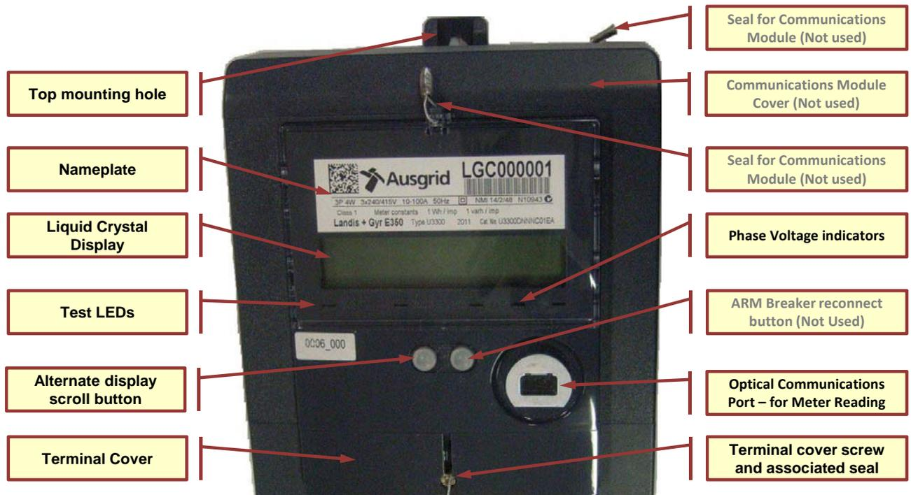
Figure 5.4-3: LGC Meter layout
