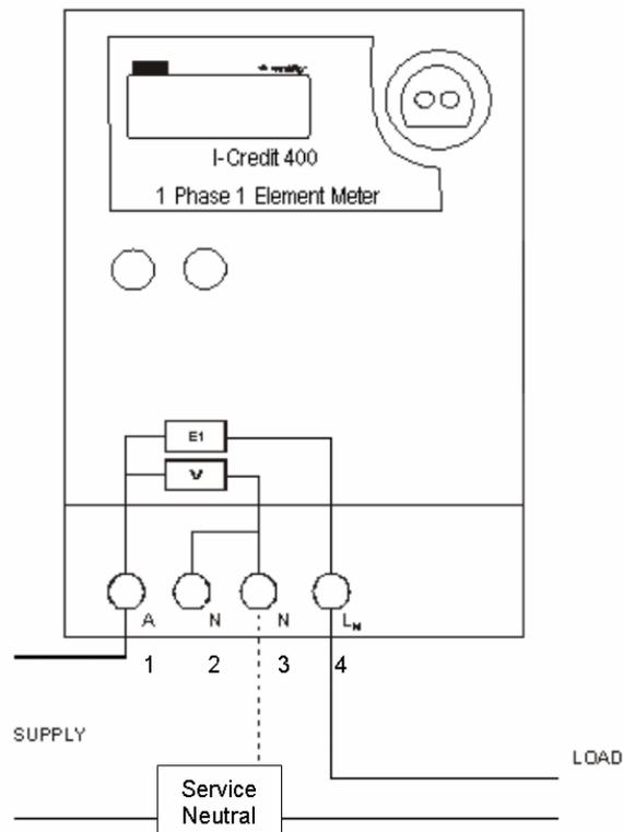
**Figure 4.2-4 i-Credit 400 meter wiring schematic**
