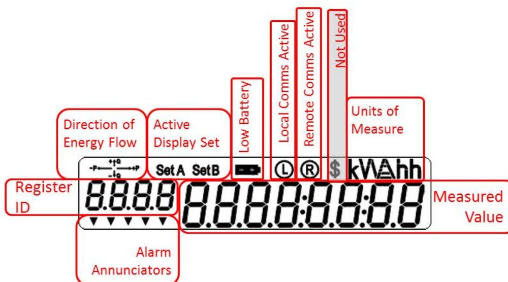
The direction of energy flow has the convention of P for Watts and Q for vars. A *plus* sign indicates energy delivered to the customer while a *minus* sign indicates energy generated by the customer.
