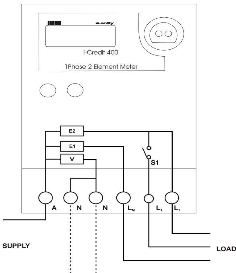
Figure 5.1-1 i-Credit 400 meter wiring schematic (configuration 210)
