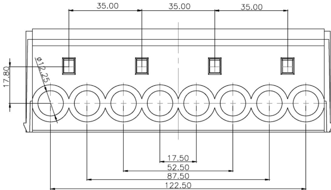
**Figure 6.1-3: EET Main Terminal Spacing**
