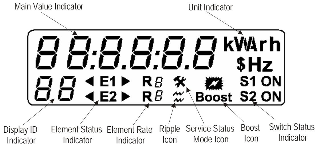
**Figure 5.1-2 i-Credit 400 meter display (Note the Boost feature is not used by Ausgrid)**
