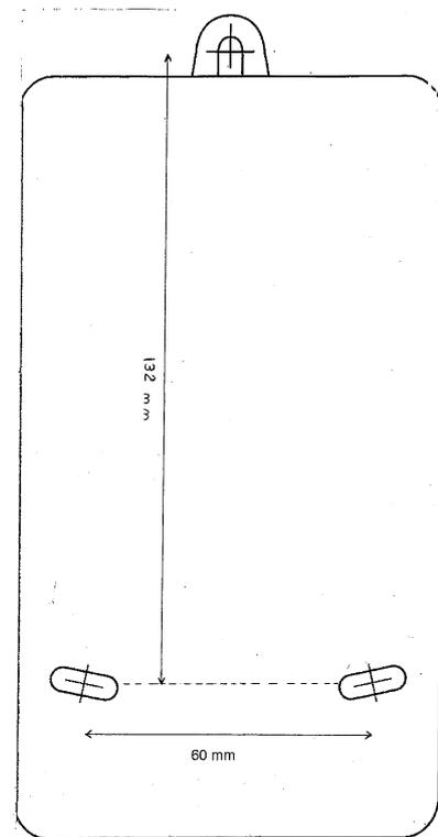
Figure 8.1-5 Drilling positions (not to scale)
