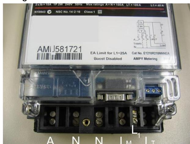
**Figure 5.2-3 Wiring terminals of AMJ**
