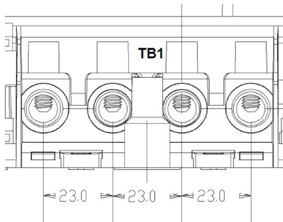
**Figure 4.3-3: EEL Main Terminal Spacing**
