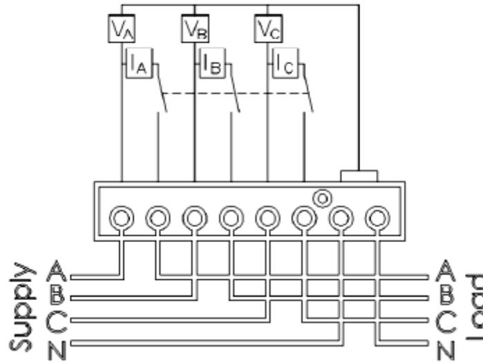
**Figure 5.4-5: LGC meter wiring schematic**
