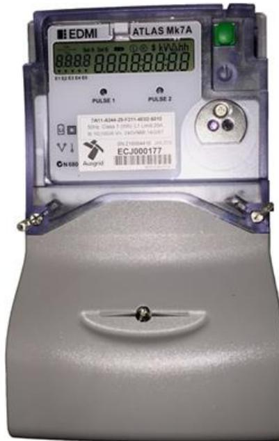
**Figure 5.3-1: ECJ meter front view**
