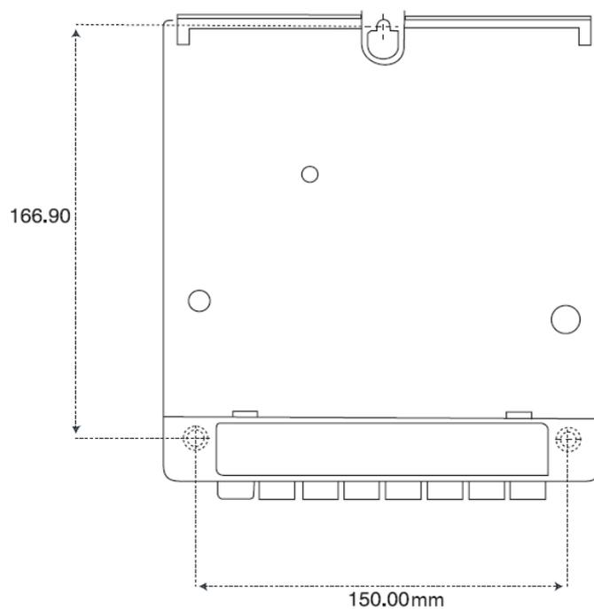
**Figure 6.2-4** Drilling Positions
