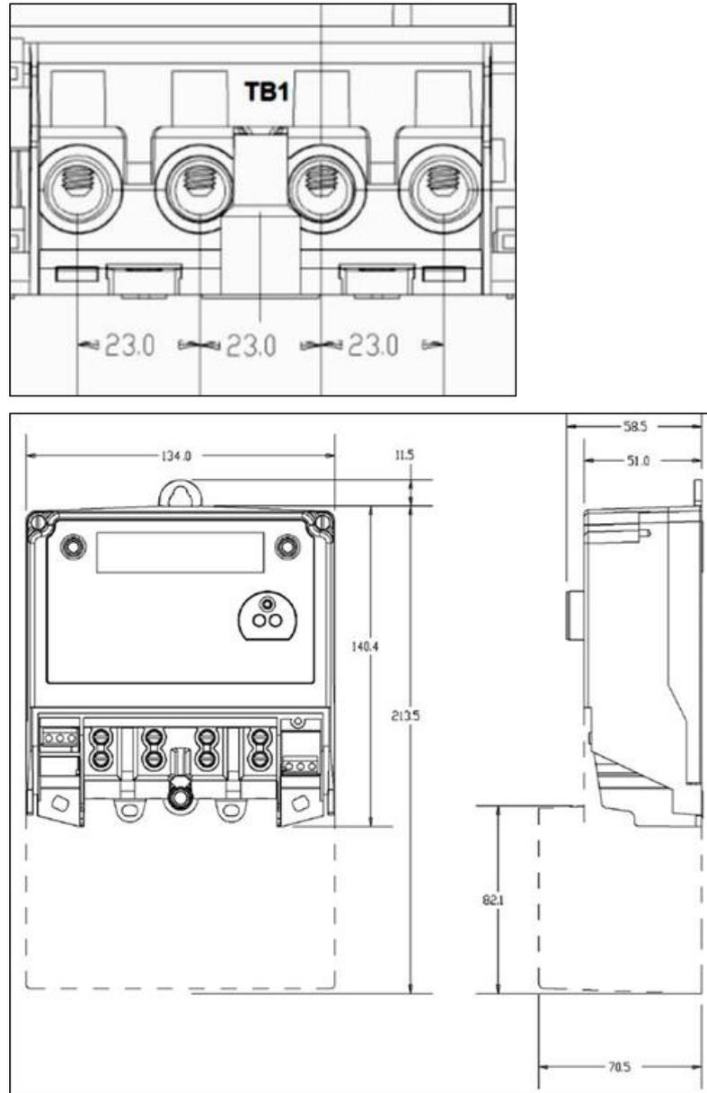
Overall height is 214mm, width 134mm and depth 70mm
