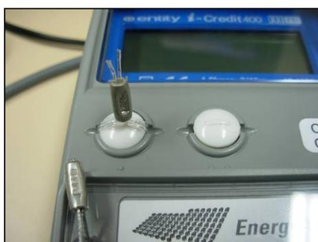
**Figure 4.2-8 Sealing the Left button**
