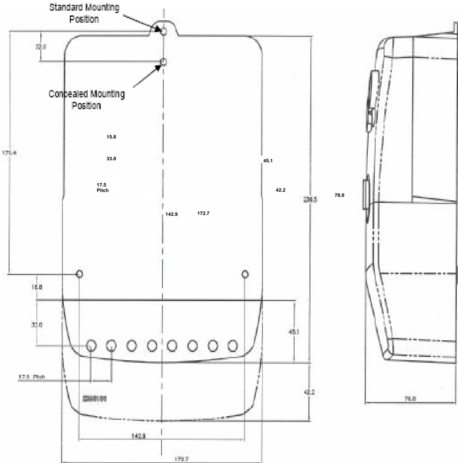
Figure 6.3-9 EM5100 meter dimensions and drilling positions (NOT TO SCALE)
