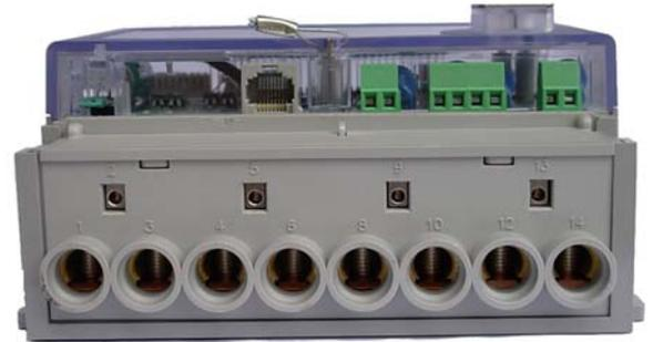
Figure 6.1-5: EET meter terminals
