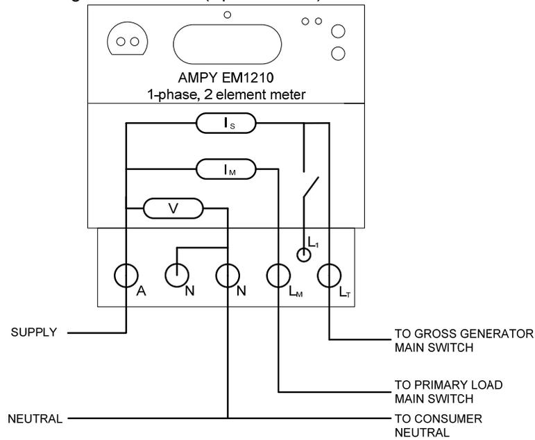
**Figure 5.2-6 Wiring Schematic for Gross Metering – Structure 26**
