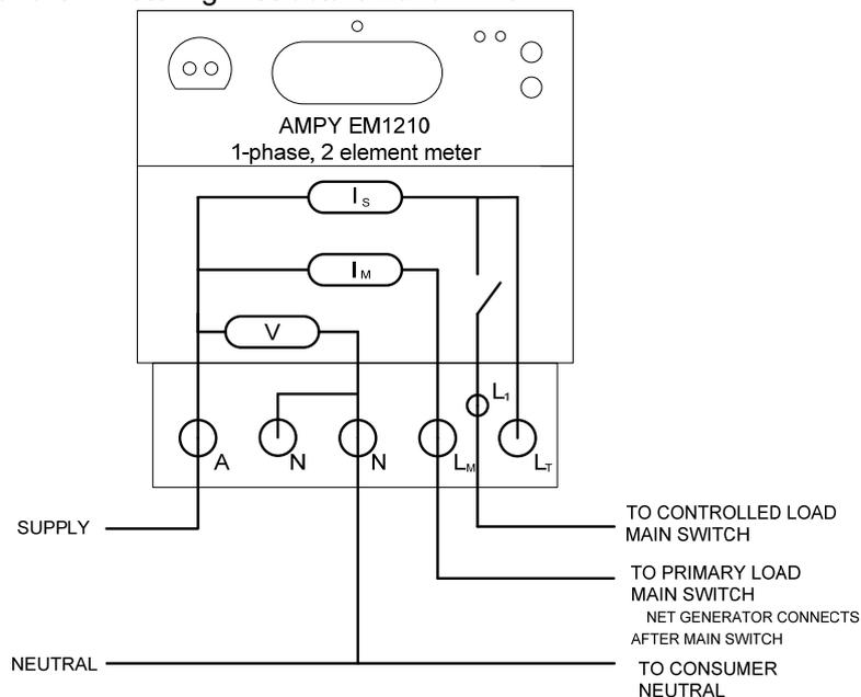
**Figure 5.2-5 Wiring Schematic for Net and OP Metering – Structure 23**
