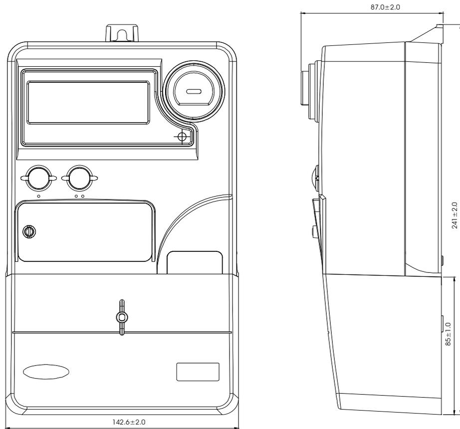
**Figure 5.1-4 Meter dimensions and mounting diagram**
