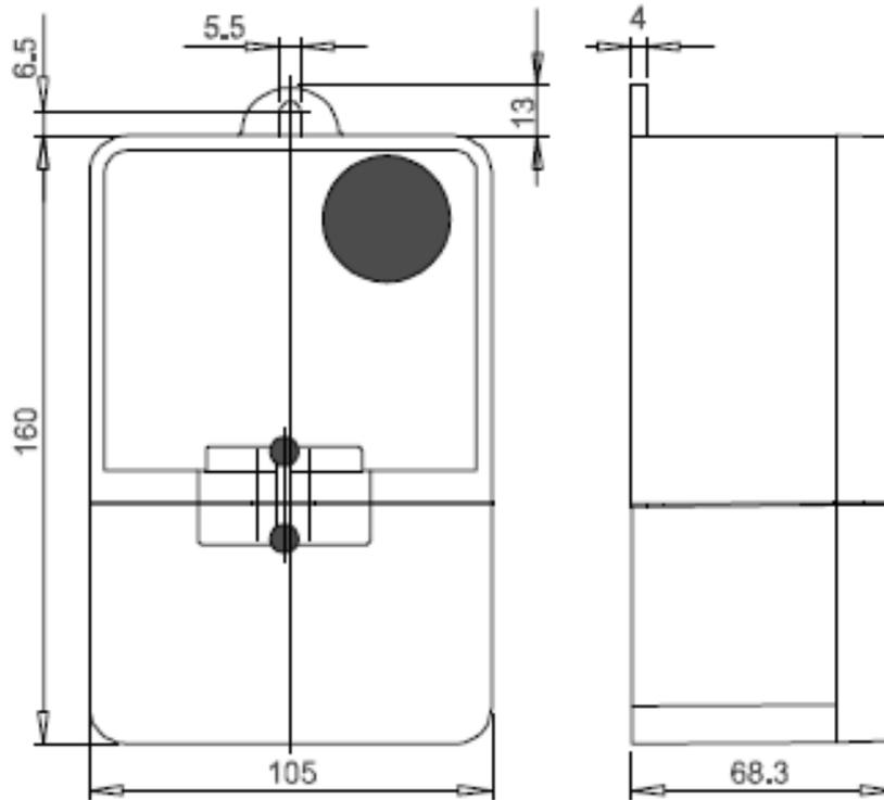
**Figure 8.2-3 Ripple Receiver Dimensions**
