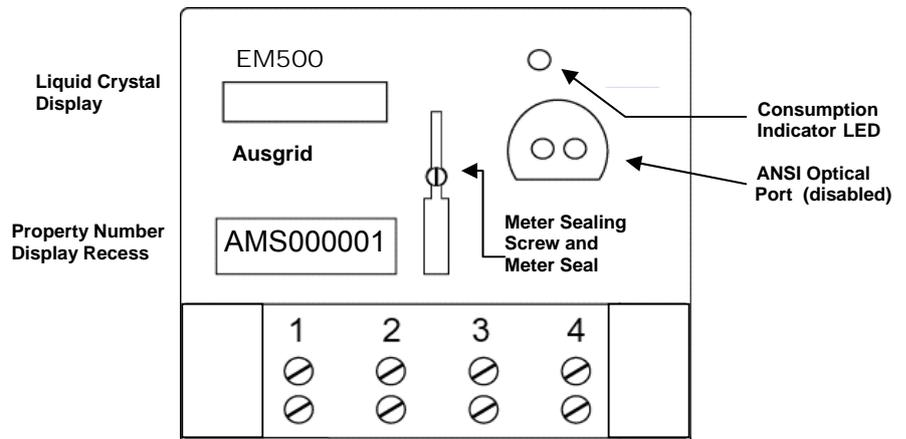
Figure 2.1-3: EM500 Meter Main Parts
