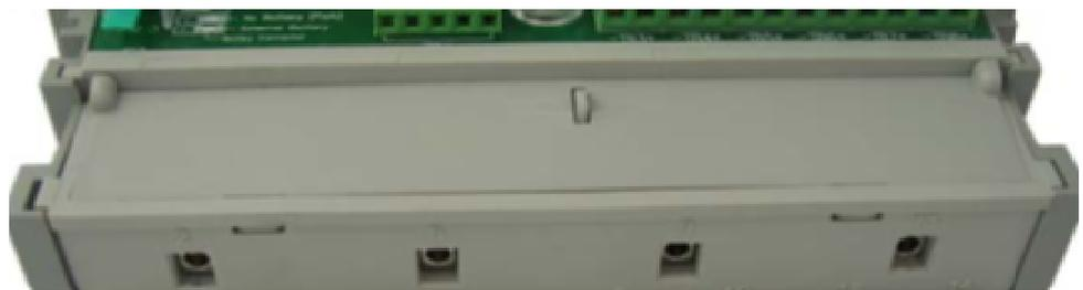
**Figure 5.5-5: ECP Terminal Finger Guard**
