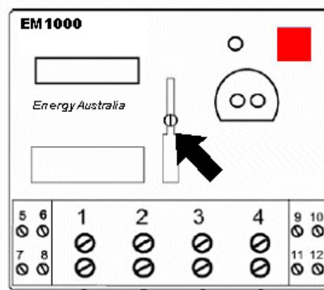
**Figure 4.1-6 EM1000 meter seal location**
