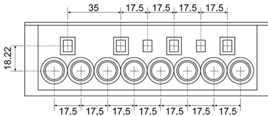
Figure 5.5-1: ECP meter dimensions (not to scale).
