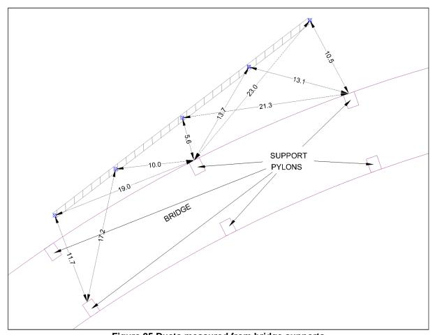
Figure 25 Ducts measured from bridge supports
