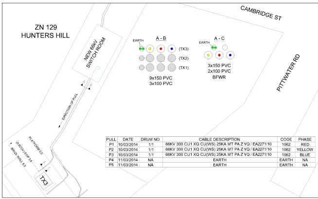
Figure 56 Drum details and direction of pull
