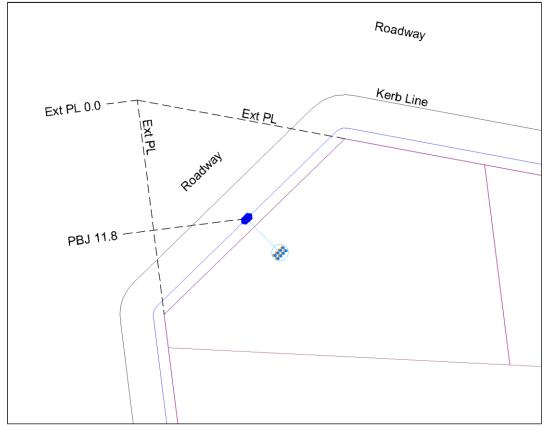
Figure 23 Extended splay runs into roadway
