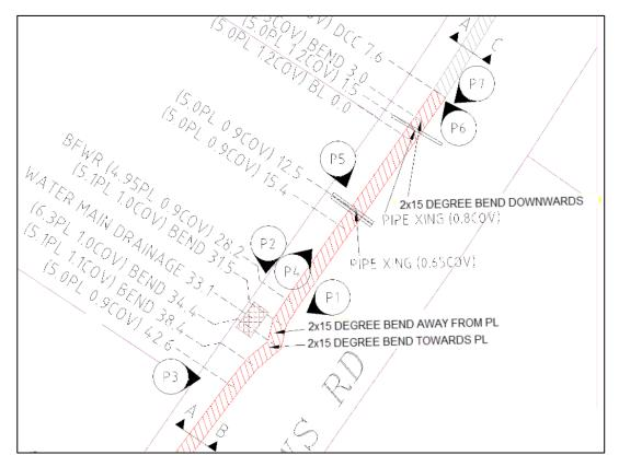
Figure 21 Linear bend changes example
