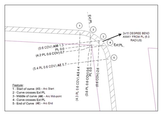
Figure 20 Measuring curves
