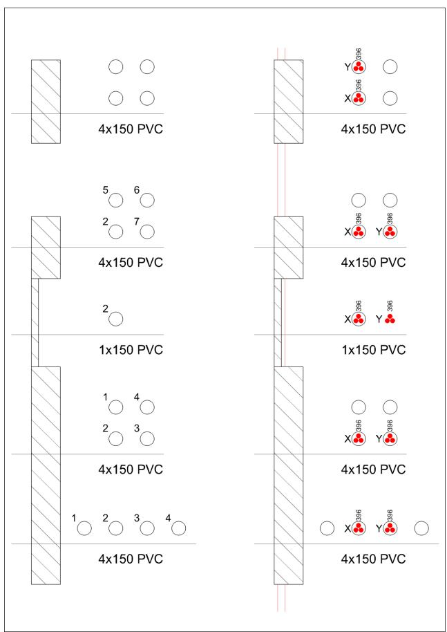
Figure 37 Example of duct numbering and cable letters
