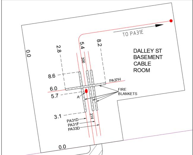
Figure 44 Example recording of fire blankets
