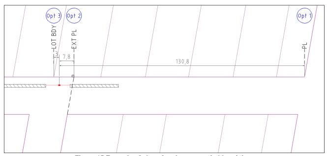
Figure 15 Example of choosing the most suitable origin
