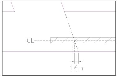
Figure 18 Measurement error when PL not extended properly
