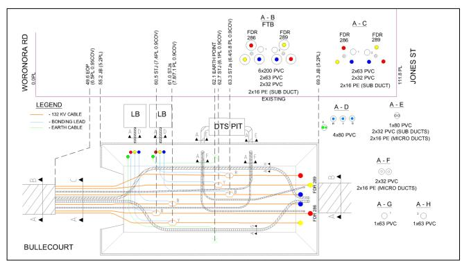
Figure 59 Example of a 132 kV joint bay
