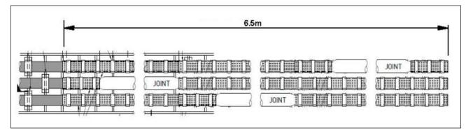
Figure 43 Example of fire blankets wrapping cables in proximity to joints
