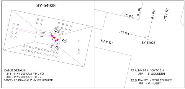
Figure 48 Jointing works in existing pit
