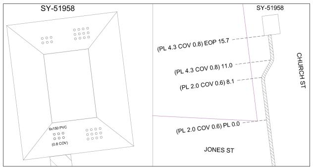
Figure 47 New ducts enter existing pit
