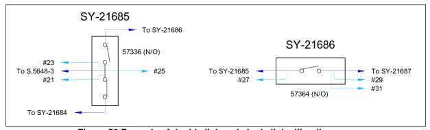
Figure 50 Example of double link and single link pillar diagrams
